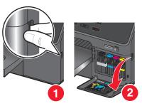
**Warning—Potential Damage:** Do not extend the ink cartridge access door beyond 90 degrees when opening to prevent it from breaking.
